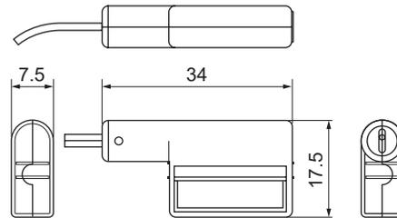
It allows you to measure the airflow condition and whether it exists. You may monitor the working status of air conditioners. Normally Closed (NC): It allows you to get in touch when airflow exists.
