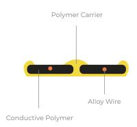
It is used for local detection of water leaks that may occur on the ambient floor. Cable options of 1, 2, 3, and 5 meters are available.
