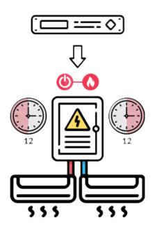
It enables 2 separate air conditioners to be operated sequentially at intervals of 12 hours a day. In the event that an air conditioner that must operate during the operating time interval fails or the system room cannot be cooled within the defined intervals, it also activates the standby air conditioner, enabling both air conditioners to be operated together and deactivating the backup air conditioner again when the system room temperature falls within the defined range.
