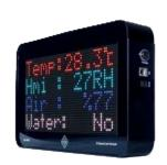
You can instantly monitor the values of sensors connected to Birsens environmental monitoring modules. There is an area of 4X10 characters on the screen that can be managed via the web interface. You can create the design you want with 7 different color support.
