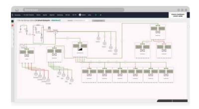
Alarms that may occur in energy monitoring can be followed instantly on the monitoring screen and the location of the fault can be easily detected from the descriptive queue address.
